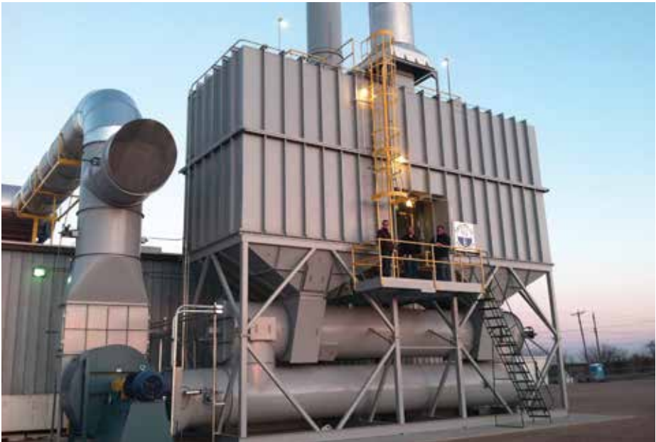
FIG. 1. Thermal oxidizers are differentiated from conventional combustors because they use excess oxygen to complete oxidation reactions at a suitably high temperature.
