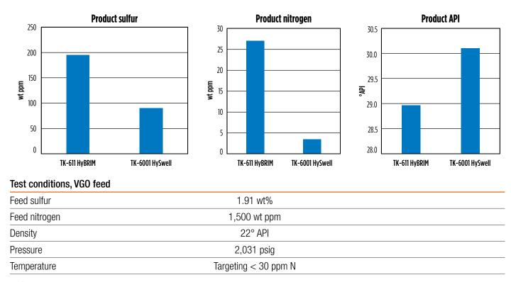
lengths. In the case of a hydrocracker, the additional activity can also be used to lower the nitrogen slip from the pretreat section to the cracking section, resulting in higher conversion and better yields. TK-6001 HySwell will also increase the volume swell due to better hydrogenation functionality, thereby creating a significant economic driver for many refineries by producing more valuable barrels.
