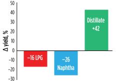
FIG. 3. The implementation of ExxonMobil's catalyst technology and optimization knowledge resulted in a 42% increase in distillate yield at constant pour point and cloud point, and a decrease in LPG and naphtha yields of 16% and 26%, respectively.
