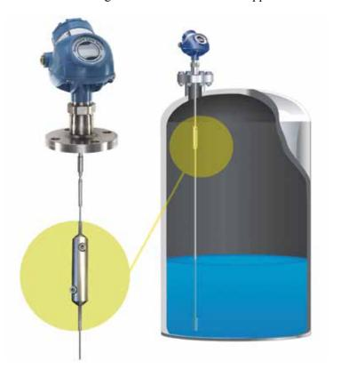
FIG. 1. A verification reflector placed on a GWR probe allows for proof testing a high level point without raising liquid levels to that point.
