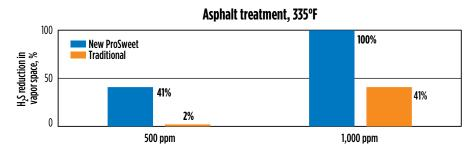
FIG. 1. Asphalt treatment results (higher is better).
