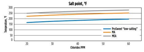
FIG. 2. Salt formation temperature curves (lower is better).
